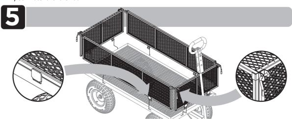
• Secure the 4x Levers to the Front and Rear Panels with the washer and nut. **Do not tighten**.
