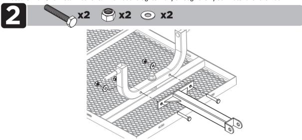
• Attach the T-Frame to the Front U-Frame with 2x M10x55 Bolt, 2x Φ10 Washer & M10 Nut. Fully tighten through the nylock material of the Nut.
